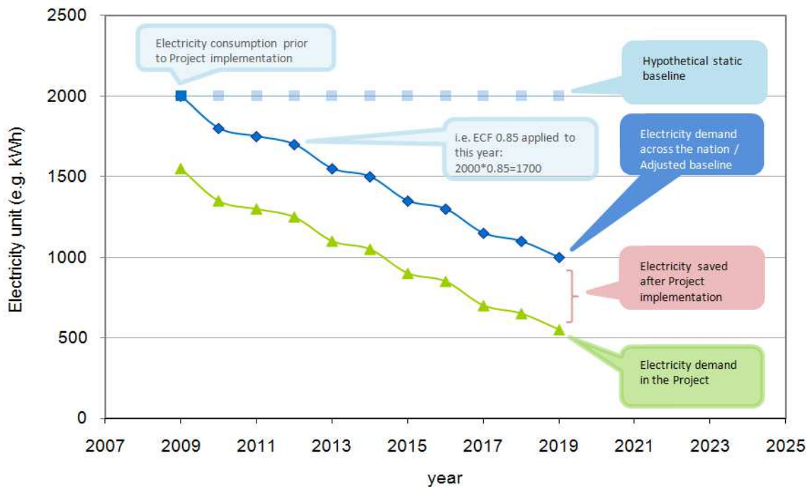
Figure 4. Reduction in electricity consumption as a result of an adjusted consumption approach
